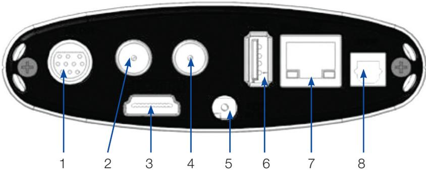
1. **Audio Visual Out** (Composite Video and Stereo Audio) Connects the set top box to your TV or VCR to provide good quality video and stereo audio - custom Amino cable has 10-pin connector at set top box end and yellow, red and white RCA connectors at TV/ VCR end. **Network** Connects the set top box to the video service using a CAT5 Ethernet cable.
