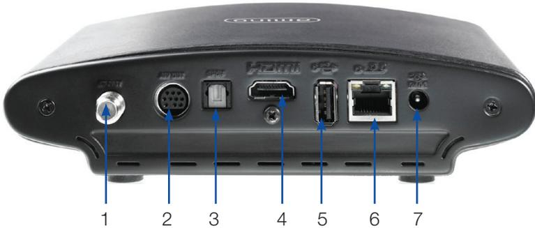
1. **Out** Connects the set top box to the TV using a standard coax cable - provides video and audio.
