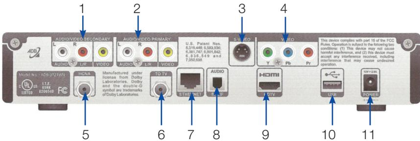
1. **Secondary Video/Stereo Audio R/L (Video/Audio Left/Audio Right)** Connects the set top box to your TV or VCR to provide good quality video and stereo audio.
